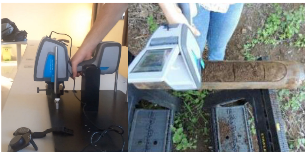
Figure 30: Pictures of the portable mid-infra-red (MIR) spectrometer
