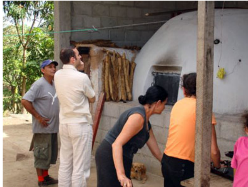
Luzi Hugentobler, Swisscontact's director of Central American operations, checks an oven used for cooking rosquillas, a bakery product made of maize and cheese, in Danli, Honduras. The new oven's separate feeding system and insulation helps to save more than 50 percent of wood. Photo by: Luzi Hugentobler
